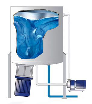
The intense high shear exerted on the polymer by the bottom entry and In-Line mixers ensures that particle size is minimised, exposing a greater surface area of polymer to the surrounding oil, allowing rapid solubilisation to be achieved. Samples can be drawn off to check dispersion and solubilisation is complete before the finished product is discharged.
