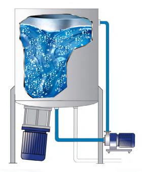
Once the solids have been reduced to granular size the Silverson In-Line mixer is started. The product is drawn from the vessel and processed in the rotor/stator workhead of the In-Line mixer before being returned to the vessel by the self-pumping action of the In-Line mixer.
