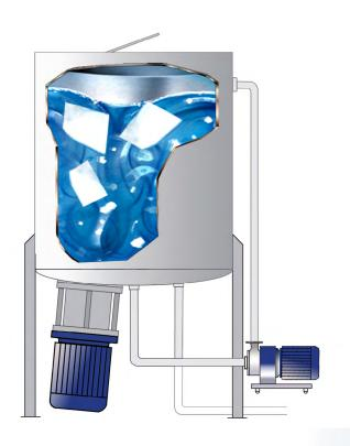
Base oil is pumped into the vessel and heated to appropriate temperature. The Silverson bottom entry mixer is started and the polymer bales are added. The powerful vortex created by the mixer draws the solids down from the surface into the coarse tooth disintegrating head of the mixer which shears off edges and corners of the bales.
